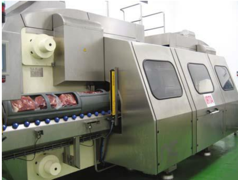
Figure 1. Industrial HHP equipment for HPP located at IRTA-CENTA (GARRIGA; AYMERICH, 2010)
